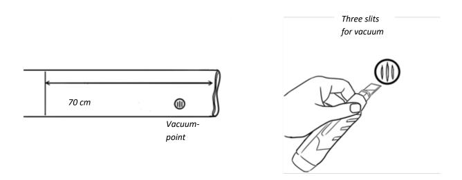
When creating the vacuum, one end is sealed with tape, and two to three cuts of 10-15 mm are made for the vacuum pump, which is connected to suck out the air. After the vacuum is achieved, the epoxy is filled into the liner while maintaining the vacuum to ensure an even distribution of the epoxy. The liner is then passed through rollers with a predetermined roller spacing adapted to the liner chosen (see table).
