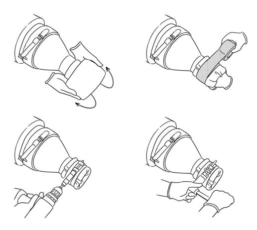
Set the extruder at an angle to the installation point and introduce inversion pressure of around 0.4–0.8 bar using a regulator. This pressure will turn the impregnated liner inside out and start the installation, which continues until the liner has reached its predetermined endpoint.
